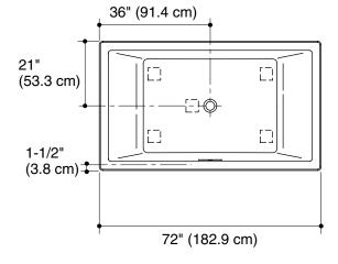
No change in measurements if connected with required drain illustrated. (K-7272)
