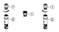
This faucet ships with a 1.8 GPM flow restrictor installed. An optional 2.2 GPM flow restrictor is also included in the box.
