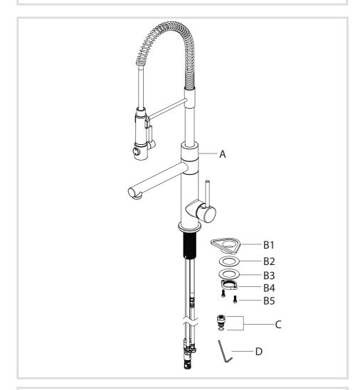
A. Faucet Body B1. Seat B2. Rubber Washer B3. Metal Washer B4. Mounting Nut B5. Screw C. 2.2 GPM Flow Restrictor D. Hex Wrench
