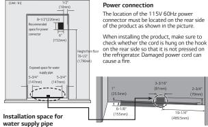
Place the water hose for ice maker and water dispenser as shown in the picture, and prepare hose to come up from the floor (Copper pipe with diameter of 5/16"(8mm) is recommended for the water hose.) If the water pipe and water hose is located far from the product, bury the water hose on the floor and provide appropriate treatment.
