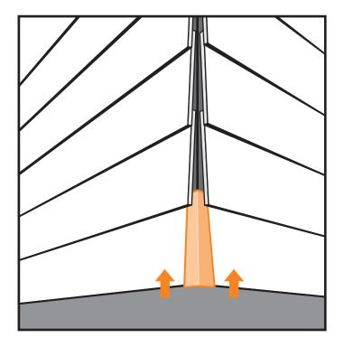
1. Start with the bottom course of siding. Carefully slide the first corner up and under the second course, and the bottom is flush to the bottom courses.
