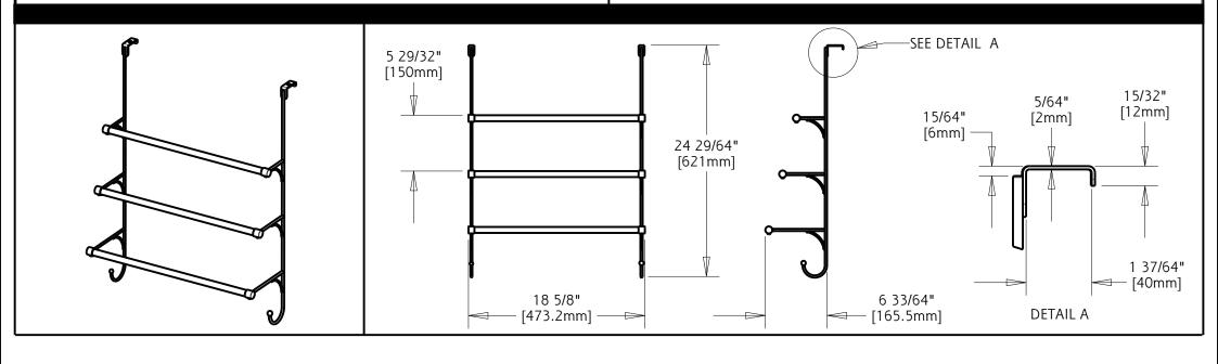
MATERIALS: Left and Right Support - Steel OTD Bracket - Steel
