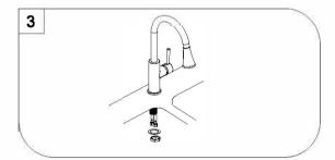
Screw the mounting stud into the body. Secure the faucet to sink by installing steel washer and nut onto it. Tighten with wrench.
