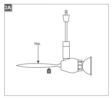
The tail can be removed for a different aesthetic. Simply unscrew the tail by hand to remove it.
