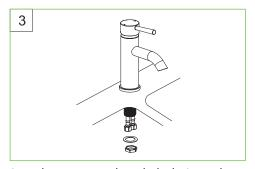
Screw the mounting stud into the body. Secure the faucet to sink/counter by installing steel washer and nut. Tighten with wrench.
