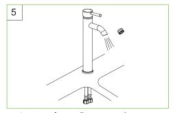
IMPORTANT: After installation is complete, remove aerator and turn on water supply and allow both hot and cold water to run for at least one minute each. While water is running check for leaks; make adjustments if necessary. Reinstall aerator. Your new faucet is now ready for use.
