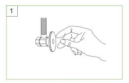
Shut off water supplies. Remove old faucet. Clean sink/counter surface in preparation for new faucet
