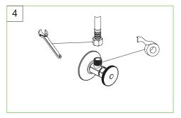
Apply pipe tape onto threads of water supplies. Use wrench when tightening the hose connection. Do not overtighten.
