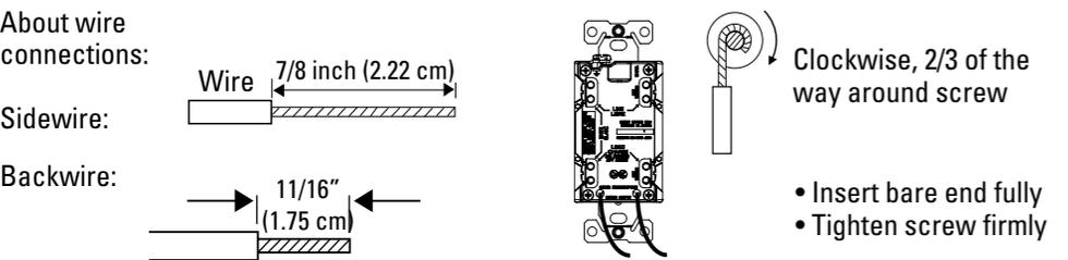
**Connect the LINE cable wires to the LINE terminals:**
