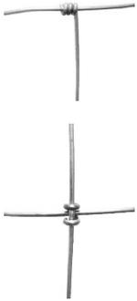
The Hinge Joint is the most common knot in agricultural fencing, found on both low carbon and high tensile products. The knot is formed by wrapping the vertical stay wire pieces around the line wire at each intersection. This design can also absorb animal impact without damage and is the most economical knot choice available. A Hinge Joint is used on the top and bottom wires of our Horse Fence.
