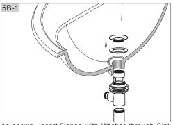
As shown. Insert Flange with Washer through Sink drain Hole. From underside, thread Drain Body into Flange. Holding the drain body in position with Ball Rod Opening facing back, tighten Metal Locknut securely. Thread Drain Tailpiece into Drain body.
