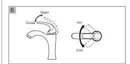
Lift the handle up, the cartridge will be activated allowing water to flow. The water flow will increase by continuing to rotate handle. By rotating the handle to the right, the water temperature will decrease to cold flow only. By rotating Handle to the left, the water temperature will increase to hot only.
