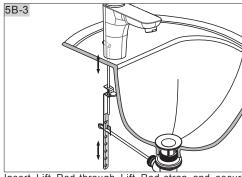
Insert Lift Rod through Lift Rod strap and secure with Set Screw. Place the Ball Rod through one of the holes on the Lift Rod Strap. Secure it with the Spring Clip. Adjust the height of the lift by resetting Set Screw. No interference between faucet and knob.
