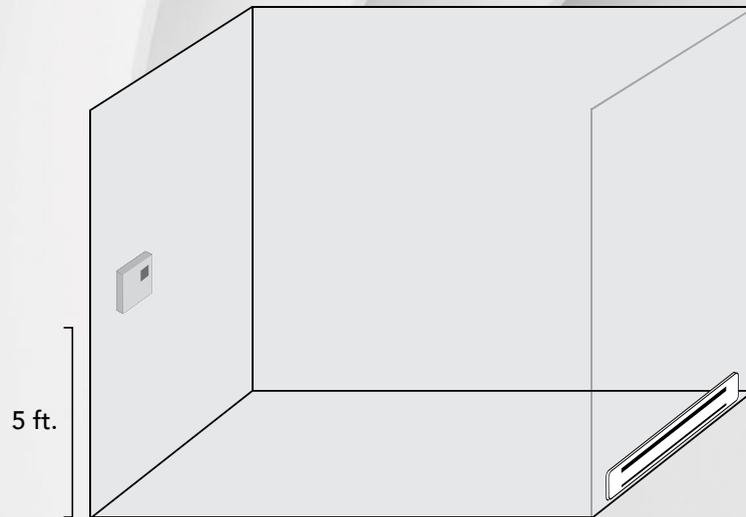
**ATTENTION:** To avoid any risk of overheating, leave a clearance of at least 12 in. around the controller•thermostat to ensure proper ventilation. Also, the front of the unit should be completely clear of any obstruction to ensure optimal functionality. For example, do not install the controller•thermostat behind curtains or furniture.
