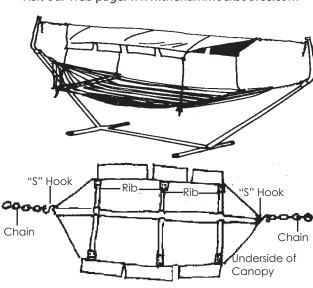
3. Position the short end (without cap) of the canopy support pole into the end of the stand pole, making sure that the holes align. Insert one end of a large "S" hook through the stand pole and the canopy support pole together to secure the canopy support pole to the stand pole.
