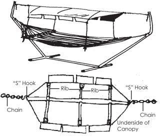
**3.** Position the short end (without cap) of the canopy support pole into the end of the stand pole, making sure that the holes align. Insert one end of a large "S" hook through the stand pole and the canopy support pole together to secure the canopy support pole to the stand pole.
