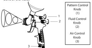
The direction of the fan (horizontal or vertical) can be adjusted by loosening the air cap ring and turning the air cap 90 degrees.
