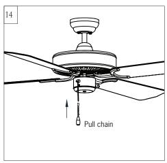
Install pull chain to preassembled pull chain on fan. Pull chains provided.
