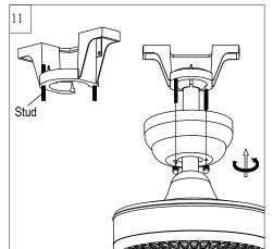
Lift Canopy allowing the 2 studs to protrude through the canopy. Next install knurled nuts as shown, knurled nuts provided. Tighten the knurled nuts securely. The canopy should adjust for any irregularity in the ceiling or Outlet box.
