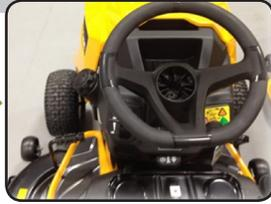
Make sure the front wheels are straight, then attach the wheel with the center line of the steering wheel facing forward and centered on the hood.
