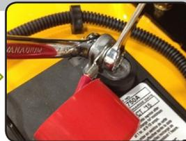
Use the 3/8" and 7/16" wrenches to attach the battery cables, the positive (red) first and then the negative (black).
