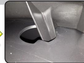
Slide the dash cover back towards the engine to lock into place. Push down in the center of the center locking tab to ensure it is hooked.
