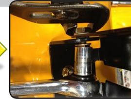
Securely tighten down the hardware using the 1/2" ratchet and channel locks (or 3/8" wrench). Tighten to 85-105 in-lbs.
