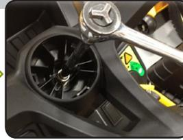
Attach the wheel using the bolt and washer. Tighten to 18-22 ft-lbs.
