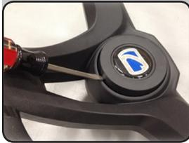
Open the wheel cover and remove the bolt and washer.
