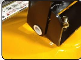
Be sure to replace the plastic clip in the seat pan before the bolts.
