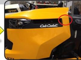
Once locked into place, check the alignment on the area circled above.
