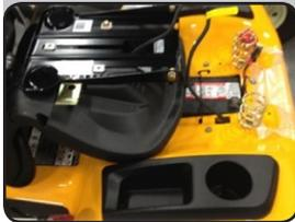
Remove the nuts and bolts on the seat pan.
