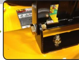
Attach the nuts and bolts with the nuts facing in.
