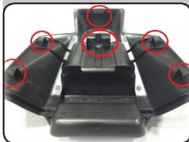
Locate the five hooks on the dash cover. And the center locking tab.
