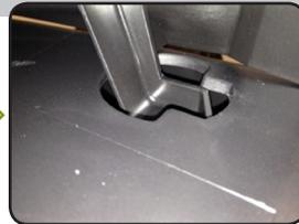
Position the five hooks into the holes on the top of the dash.
