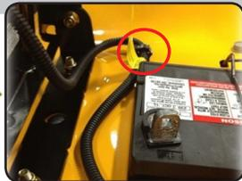
Push the clips into the body panel to lock in place.
