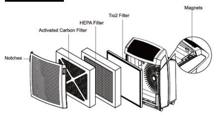
When the "HEPA" indicator lights up, it means the HEPA Filter has been used for 8000 hours and needs to be replaced.
