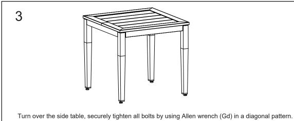
Turn over the side table, securely tighten all bolts by using Allen wrench (Gd) in a diagonal pattern. Adjust the table level by twisting knobs on the bottoms of the legs.
