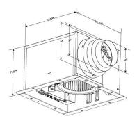
ETL/cETL Listed for installation over tub/shower enclosure when used with GFCI circuit wiring
