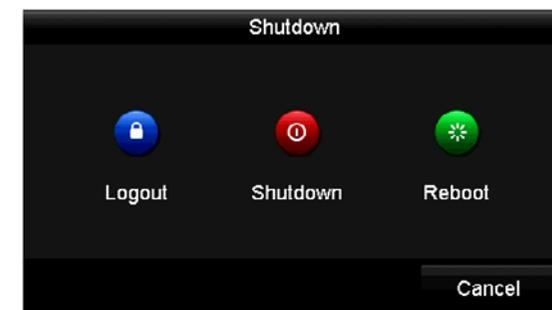
To shutdown or reboot your DVR, or simply log out of the current user account, click the "Shutdown" button. To ensure the integrity of your data and recordings, always select "Shutdown" when powering off your DVR.
