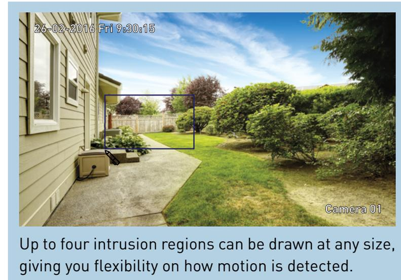
Up to four intrusion regions can be drawn at any size, giving you flexibility on how motion is detected.
