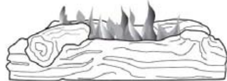
Figure 21 - Correct Burner Flame Pattern
