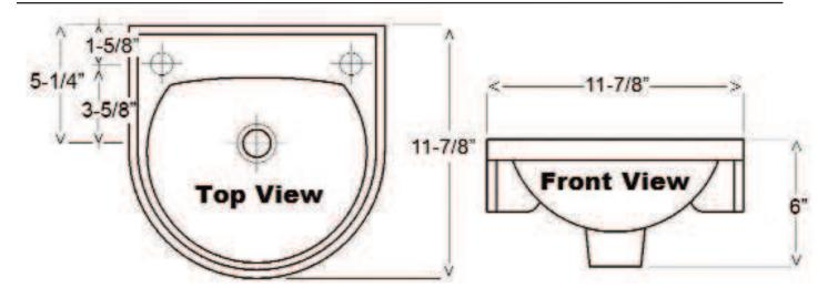
Dimensions of fixture are nominal and may vary within the range of tolerances established by ASME Standard A112.19.2. Dimensions and specifications subject to change without notice.
