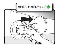
When the VEHICLE CHARGING light stops blinking on the charger, press the button on the connector to release. Pull to remove from vehicle charge port.
