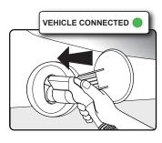
Insert connector firmly into the vehicle charge port. When fully inserted, the VEHICLE CONNECTED light on the charging dock will illuminate.
