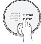
Charging will stop automatically when complete. Or, you can manually stop charging by pressing STOP. In either case, when the READY TO CHARGE light blinks, remove the connector from the vehicle charge port. If you manually paused charging by pressing STOP, you can press START to resume charging.
