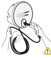
Remove the connector from the vehicle. Rewrap the charging cable around the cable hanger, and insert the Connector into the charging dock for storage.
