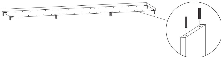
**7** Add L brackets for the top shelf, ensuring that the back of the shelf is attached to studs in the wall, and that the sides are attached into the cabinets and/or walls on either side.
