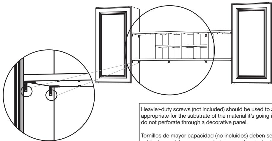
Heavier-duty screws (not included) should be used to attach brackets to walls or cabinets, and should be appropriate for the substrate of the material it's going into. CAUTION: Take care that longer screws, if used, do not perforate through a decorative panel.
