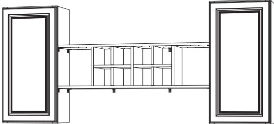
**2** Starting with the long 48" horizontal panel, use this as the lower base shelf, and find the bottom measurement where shelf will sit, aligning it with adjoining cabinets or walls.
