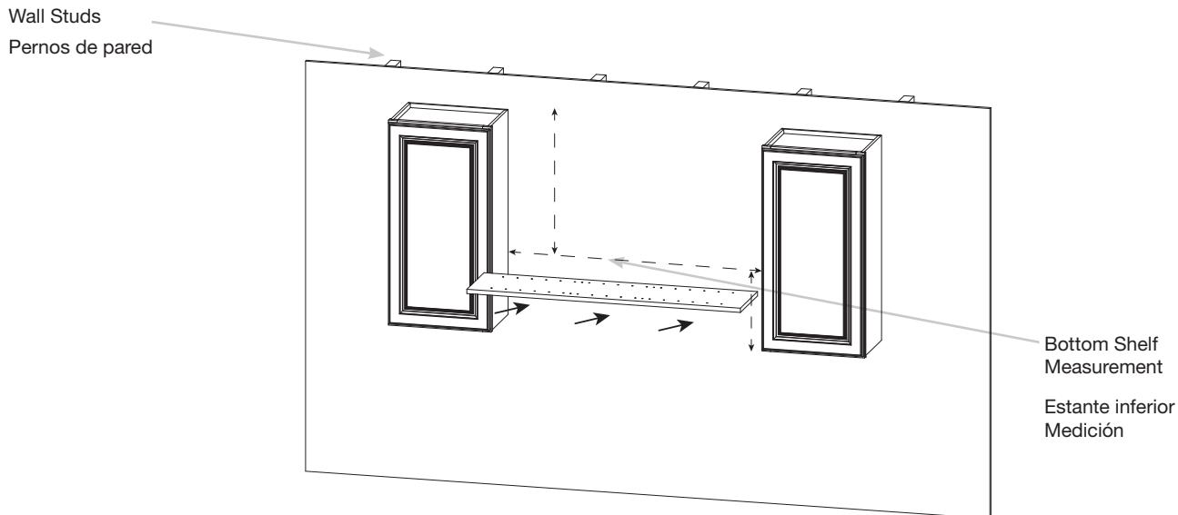
**Locate studs; attach the shelf with the provided L brackets in two places along the back, into the studs. Attach the ends of the shelf, using L brackets, into either cabinet or wall, on either side, so this bottom shelf is completely anchored on both sides and back.**
