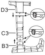
□ Insert the section 5 of E (E3) into the section 4 of E (D3). Insert the section 6 of E (F3) into the section 3 of E (C3). Secure with plastic ties (DD).
