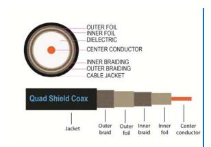
Ouad cable has an extra foil and extra braid layer, making the cable thicker than standard dual/regular RG6 cable.
