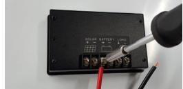
Step 4: Attach the lug end of the red cable to the positive terminal on the battery. Attach the lug end of the black cable to the negative terminal on the battery. If your battery has sufficient charge (11.5 volts or more), you should now see the LCD display light up on the controller. This means the controller has power (controllers are powered by the battery, not the panels).
