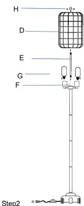
Insert the Harp (E) into the Metal cap (F).
