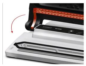
5. Firmly press the cutter arm down over the bag roll where you'd like to make the cut. Then move the slider on top of the cutter arm across the bag roll to make the cut.
