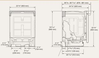
Water supply hose, drain hose and electric cable should be passed through this area
