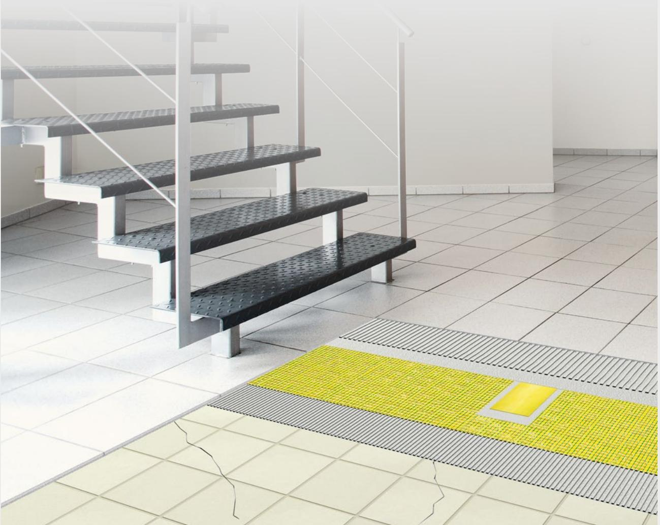
With its triple-layer construction, the multifunctional DURABASE CI++ matting system offers so much more than simply decoupling. The crack-bridging properties of the mat and its optimised shear force protection enable new tiles to be laid on old and damaged tiled floors, provided that these are still load-bearing.
