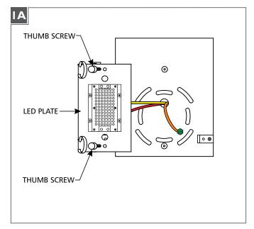
To gain access to the mounting plate holes, remove the two thumb screw to temporarily loosen the plate holding the LED lamp.
