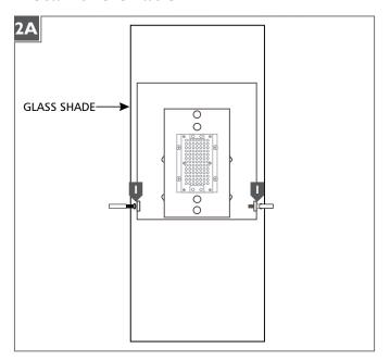
Align the holes in the glass shade with the mounting plate and screw in the thumb screws completely.
