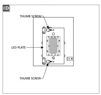
Re-install the LED Plate and secure it tightly with the two thumb screws.
