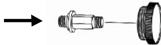
Figure 11 - Turning Pressure Selecting Screw Over/Attaching to Regulator Cap – LP/Propane Gas Position
