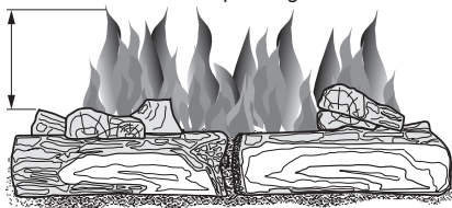
Figure 27 - Incorrect Burner Flame Pattern
