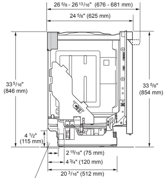
Water supply hose, drain hose and electric cable should be passed through this area.
