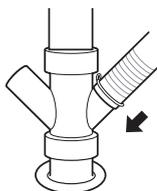
**Connecting to Disposal or Waste Tee with Air Gap**
