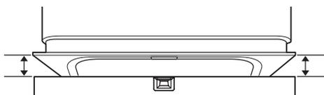
The water level should be checked after the initial fill on the Normal cycle. If the water level is not near the center of both tub lower indentations, the dishwasher may not be correctly leveled. The dishwasher may leak during operation if it is not correctly leveled.
