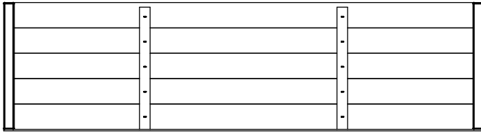
(1) RP3 - ROOF PANEL - W2A01862 1 3/8"x16 1/8"x59 1/2" (35x410x1532)
