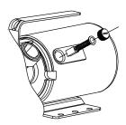
The brush must enter the square hole. Match the brush curve to the armature curve. If there are any damages to these parts, please contact the pump experts at 1-844-241-5521.
