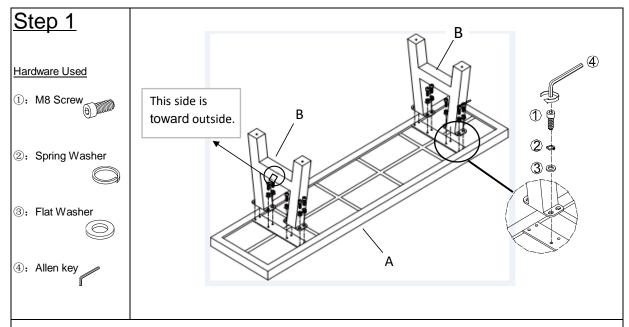
Position the bottom of the Bench top(A) as shown.
