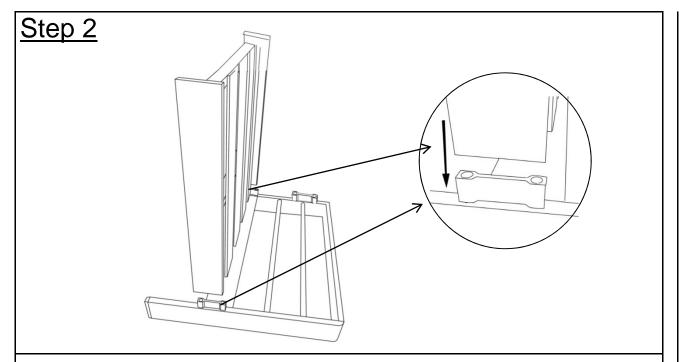
Insert the Seat(C) onto the Side Panel(A), as shown in the picture.
