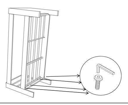
Repeat Step 1 to Step 3 to attach the second Side Panel(A). Loosely tighten the Bolts.
