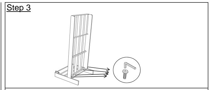
Attach Seat(C) and Side Panel(A) using Bolt(D) and Allen Key(E). **Loosely tighten the Bolts.**
