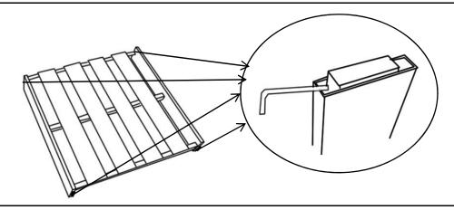
Take out the silders in the four ends of the Seatboard(C) using Allen Key(E).
