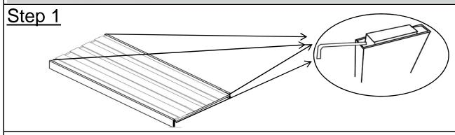
Take out the silders in the four ends of the Seatboard(C) using Allen Key(E).
