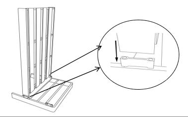
Open the carton and place all the parts on a clean, non-marring surface. Insert the Seat(C) into the Side Panel(A), shown as the picture.
