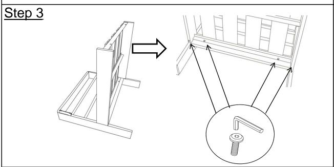
Attach Seat(C) and Side Panel(A) using Bolt(D) with Allen Key(E) as shown in the picture. **Loosely tighten the Bolts.**
