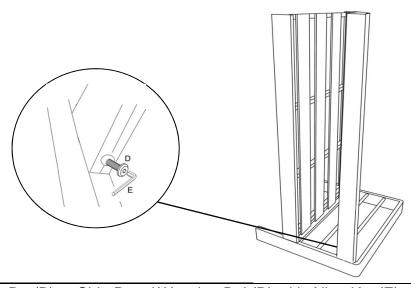
Attach Back Support Bar(B) to Side Panel(A) using Bolt(D) with Allen Key(E). Loosely tighten the Bolt.
