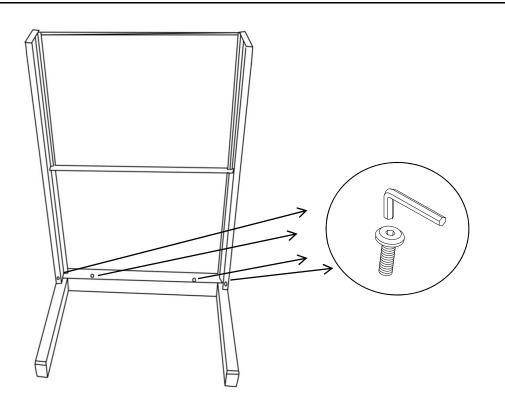
Open the carton and place all the parts on a clean, non-marring surface. Attach the Table Top Frame(C) to the Left Leg(A) using Bolt(E) and Allen Key(F) as shown in the picture.
