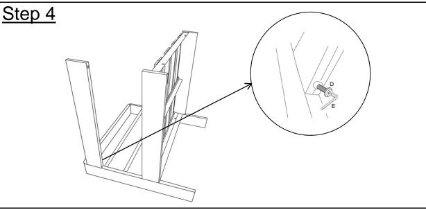
Attach Back Support Bar(B) to Side Panel(A) using Bolt(D) with Allen Key(E). **Loosely tighten the Bolts.**
