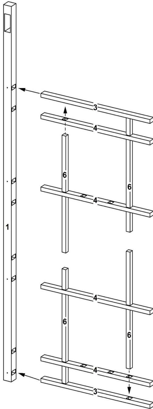
Starting at bottom of one 84" left post (part 1), insert one 27½" outer cross rail (part 3) and two 27½" inner cross rails (part 4). When inserting two inner cross rails insert sides with four routed holes facing each other. Insert two 26½" vertical rails (part 6) through outer holes of inner cross rails and into outer holes of outer cross rail.
