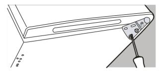
6. Screw the bottom hinge into place on the new side. Replace the foot on the other side.
