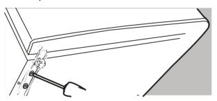
7. Check that the door is aligned horizontally and vertically and that the seals are closed on all sides before finally tightening the bottom hinge. Readjust the leveling feet.
