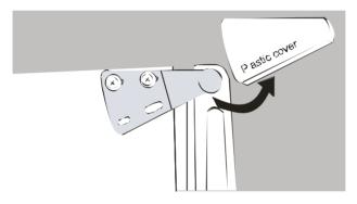
5. To install the bracket on the left side of the appliance, screw the two screws through the bracket and into the top of the appliance. Slide the door back on to the top hinge. Ensure the door is face up. Replace the plastic cover on the top bracket by pressing down until it clicks into position.
