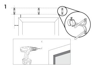
Place brackets against wall or ceiling at desired locations and mark at the top of the screw holes. Use tape measure and level to make sure marked screw holes are horizontal to each other.
