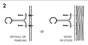
For mounting to drywall or paneling, pre-drill two pilot holes for each bracket (1/4" drill bit) and insert anchors into wall and insert screws into wall anchors. For mounting directly into wood or studs, wall anchors will not be necessary.
