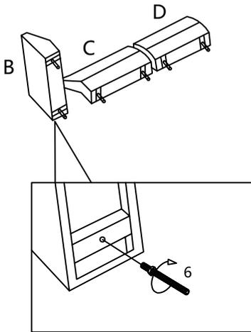
STEP 2 - MOUNT BACKS & ARM INTO THE SEAT FRAME
