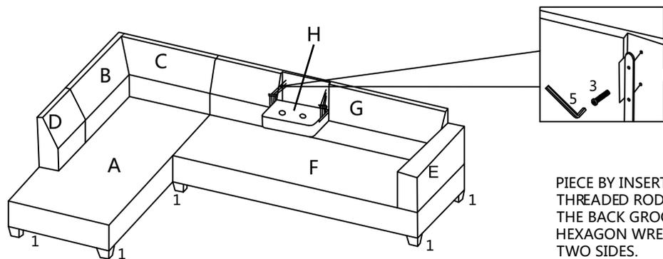
PIECE BY INSERTING THREADED RODS INTO THE BACK GROOVE WITH HEXAGON WRENCH AT TWO SIDES.
