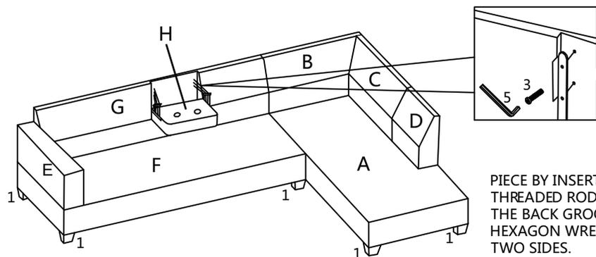
PIECE BY INSERTING THREADED RODS INTO THE BACK GROOVE WITH HEXAGON WRENCH AT TWO SIDES.
