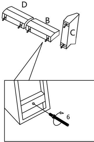
STEP 2 - MOUNT BACKS & ARM INTO THE SEAT FRAME
