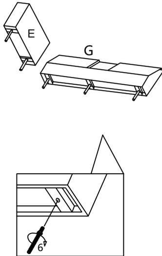
STEP 2 - MOUNT BACKS & ARM INTO THE SEAT FRAME
