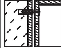
**CONCRETE:** Drill 1/4" holes, insert #10 wall anchors and secure to wall with #10 x 3" screws.
