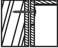
**STUDS:** Secure to wall with #10 x 3" screws at stud location.
