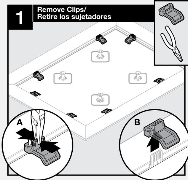
Pinch tabs to release from locking position and lift up./
