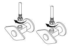
Attach waterlines to angle stops and tighten until snug. Turn on angles stops and check for leaks (DO NOT TURN FAUCET ON)
