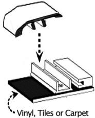
**Multipurpose Reducer (MPR)** is 72" long and transitions flooring of different heights. For example, from carpet to vinyl.
