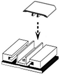
**T-Molding (T)** is 72" long and transitions different types of flooring of the same height. For example, vinyl to vinyl.
