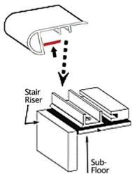
**Overlap Stairnose** is 94" long. Existing tread bullnose must be cut off.
