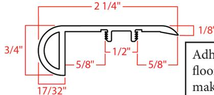
Adhere a 3/8" wide piece of vinyl floor being installed under nosing, making it even and secure.
