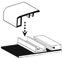
**Carpet Reducer/Baby Threshold** is 72" long and transitions flooring of different heights. For example, from carpet to vinyl. Works with sliding glass doors and fireplaces.
