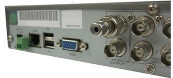
**Plug RCA cable to BNC connector**
