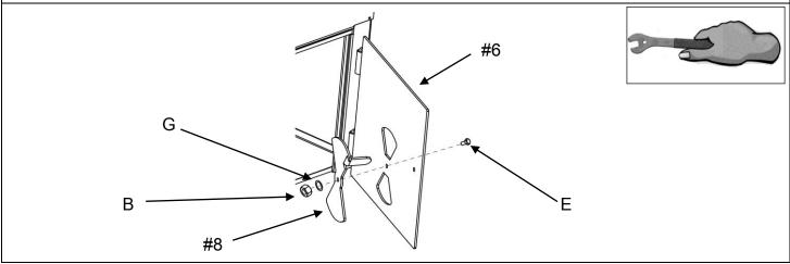
Step 16. Assemble Firebox Door Handle (Part #7) using 1 pc of Shoulder Bolt M8 x 18 (E) and 1 pc of Lock Nut M8 (F) on Firebox Door (Part #6)
