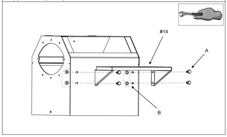
Step 13. Assemble Firebox Lid Support (Part #3) using 2 pcs of Bolt M8 x 16 (A) and 2 pcs of Nut M8 (B) on Firebox (Part #5)
