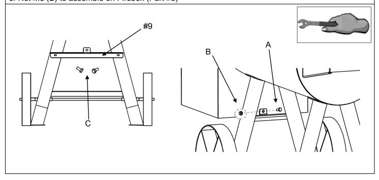
Step 12. Assemble Firebox Front Table (Part #14) using 4 pcs of Bolt M8 x 16 (A) and 4 pcs of Nut M8 (B) on Firebox (Part #5)
