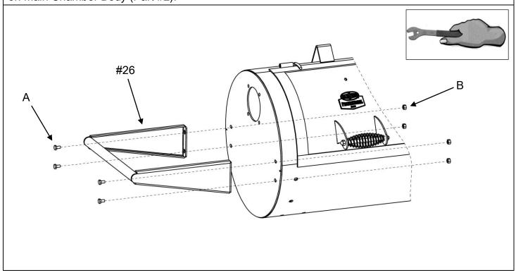
Step 6. Assemble Smoke Stack (Part #27) using 4 pcs of Bolt M8 x 16 (A) and 4 pcs of Nut M8 (B) to Main Chamber Body (Part# 2)
