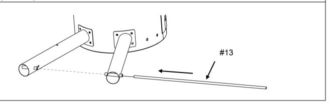
Step 3. Insert Wheels (Part #12) through Axle (Part #13) and lock with 2 pcs of Lock Nut M12 (D)
