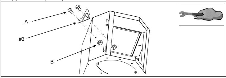
Step 14. Assemble Firebox Lid (Part #4) using 1 pc of Bolt M5 x 10 (I) and 1 pc of Washer M6 (H) on Firebox (Part #5)
