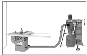
Keep hoses and ducting safely mounted along the walls.
