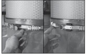
**10.** Use the belt clamp to hold the bag in place, making sure the metal strap is sitting in the groove on the lower portion of the canister.
