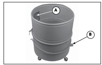
5. Set the upper drum on the lower drum, positioning the window **A** opposite the tube **B**.
