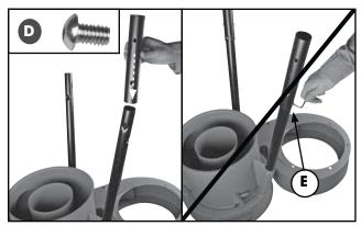
Slide a connector onto each leg, align its mounting holes with the corresponding holes in the leg, then secure the connector with 3 cap screws D per connector using a 5 mm Allen key.
