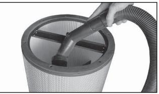
*For a more thorough cleaning*, after rotating the handle, detach the canister and place it on the ground. Vacuum the inside of the canister to remove any remaining dust from inside. Re-attach the canister and re-install its collector bag.
