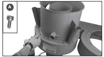
3. Attach the cyclone to the impeller using 12 cap screws **A** and a 4 mm Allen key.
