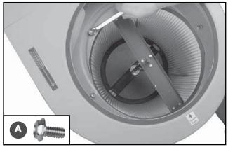
2. Align the canister mounting holes with the corresponding holes in the impeller, then attach the cansiter with 6 flange bolts **A** using a 12 mm wrench.
