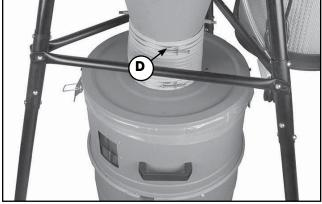
16. Verify that the junction hose has been cut to the correct length by placing the drum under the lid. Then remove the drum and detach the hose with the lid from the cyclone by loosening the hose clamp D.
