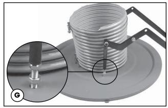
**18.** Hand tighten the bolts in the threaded ends of the quick-remove handle draw bars **G**.
