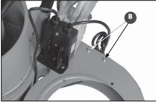
1. Using a 10 mm wrench remove the 2 flange bolts B.
