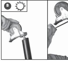
Screw the lockable swivel caster with a sprocket washer B into the short leg, then secure it in position by tightening the two jam nuts using two 14 mm wrenches.
