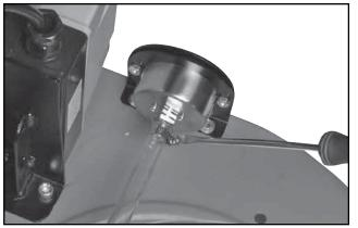
**4.** Slide the hose onto the gauge inlet, then tighten the hose clamp using a flat screwdriver.
