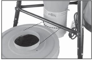
14. Place the drum against the junction hose to evaluate if the hose needs to be cut. Make a reference mark and cut as needed.
