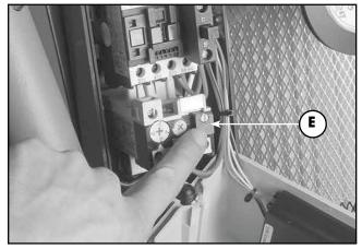
Press on the button E to reset the overload protection. Re-install the cover and then retighten the two screws D before starting the machine.
