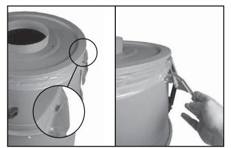
**10.** Place the lid on the drum making sure the hooks are aligned with the latches. Secure the drum lid by clamping the latches.
