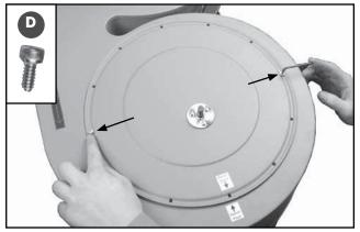
6. Align the lid mounting holes with the corresponding holes in the impeller, then secure the lid by starting with screws **D** on opposite sides.
