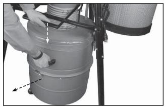
**22.** Lower the handle to lift the lid and confirm that there is enough space between the lid and the drum to remove the drum easily.
