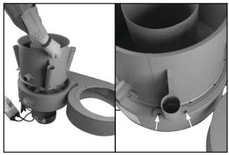
2. Place the upper cyclone on the impeller and align its mounting holes with the corresponding holes in the impeller separator.
