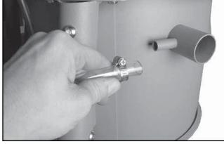
1. Slide a small hose clamp onto the pressure gauge, and slide the hose onto the fitting at the rear of the impeller.
